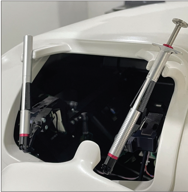
Figure 3: The multi-purpose handpieces on the HelpMeSee eye surgery simulator which are used to navigate the 'virtual instruments' in the eye on the simulator and provide real-time haptic feedback
