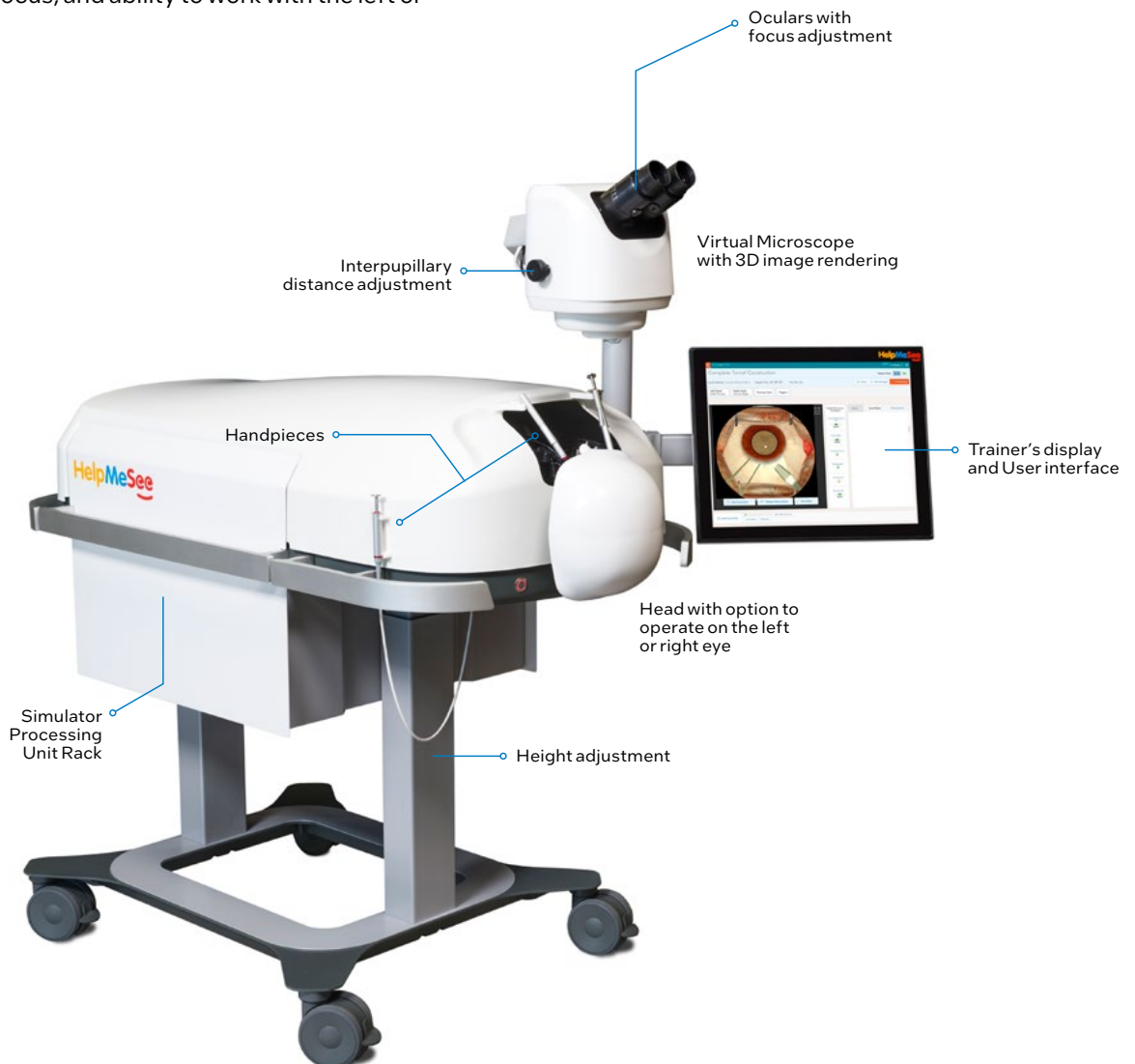
Figure 3. Eye Surgery Simulator hardware (courtesy HelpMeSee).
