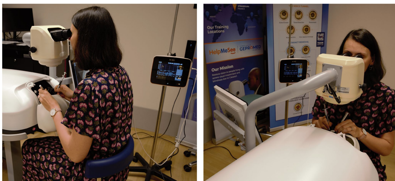
FIGURE 1 Set up of the simulation sessions. Participant performing the simulation session in a dedicated room on the HelpMeSee simulator with two electrodes (one on the right shoulder, the second at the apex of the heart) plugged to the Analgesia Nociception Index (ANI) monitor for instantaneous acquisition as a function of time over the whole simulation session.
